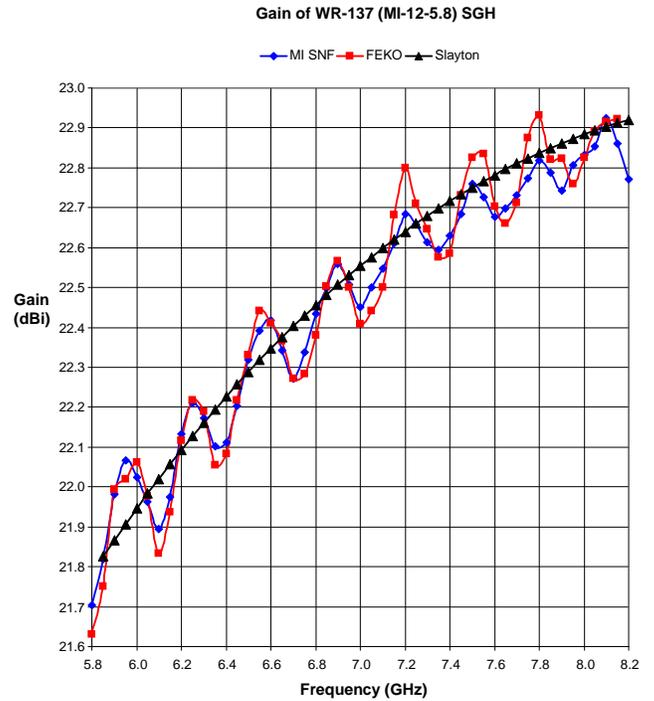
Figure 2. Calculated versus measured gain of a WR-137 standard gain horn.
