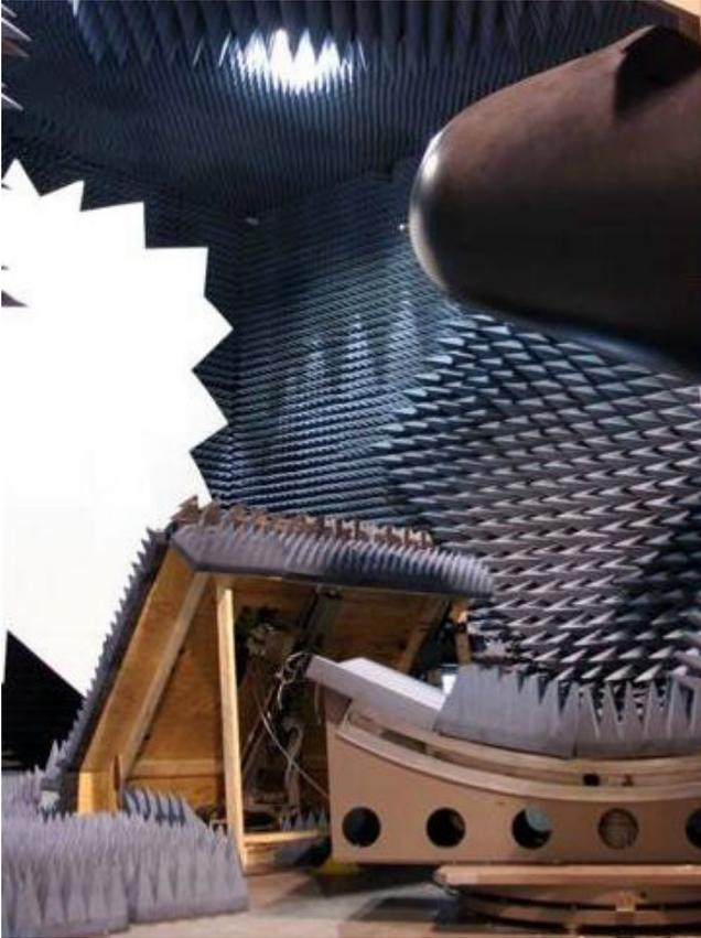
**Figure 4 – Rear View of Focal-Plane Scanner**
