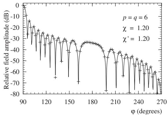
**Figure 11** - H-plane pattern. Solid line: exact. Crosses: reconstructed from NF measurements.
