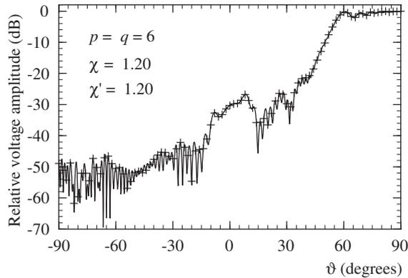
**Figure 4** - Amplitude of  $V'$  on the meridian at  $\varphi = 90^\circ$ . Solid line: exact. Crosses: interpolated.
