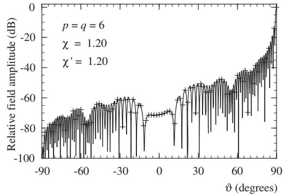
**Figure 10** - E-plane pattern. Solid line: exact. Crosses: reconstructed from NF measurements.
