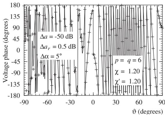
**Figure 9** - Phase of  $V'$  on the meridian at  $\varphi = 90^\circ$ . Solid line: exact. Crosses: interpolated from error affected data.
