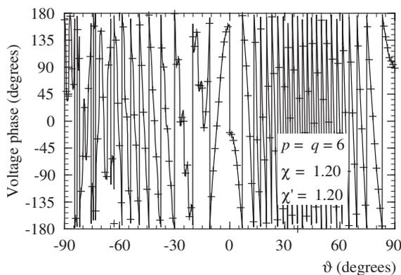
**Figure 5** - Phase of  $V'$  on the meridian at  $\varphi = 90^\circ$ . Solid line: exact. Crosses: interpolated.
