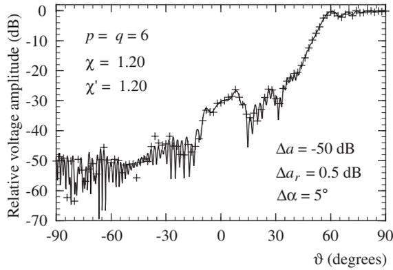
**Figure 8** - Amplitude of  $V'$  on the meridian at  $\varphi = 90^\circ$ . Solid line: exact. Crosses: interpolated from error affected data.
