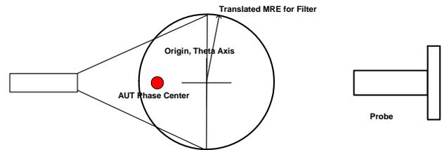
**Figure 12** Schematic for the aperture of a pyramidal horn translated to the origin of the coordinate system.
