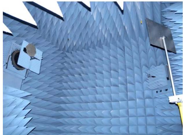
**Figure 5** – 2'x2' Metal Plate Obstruction in Chamber
