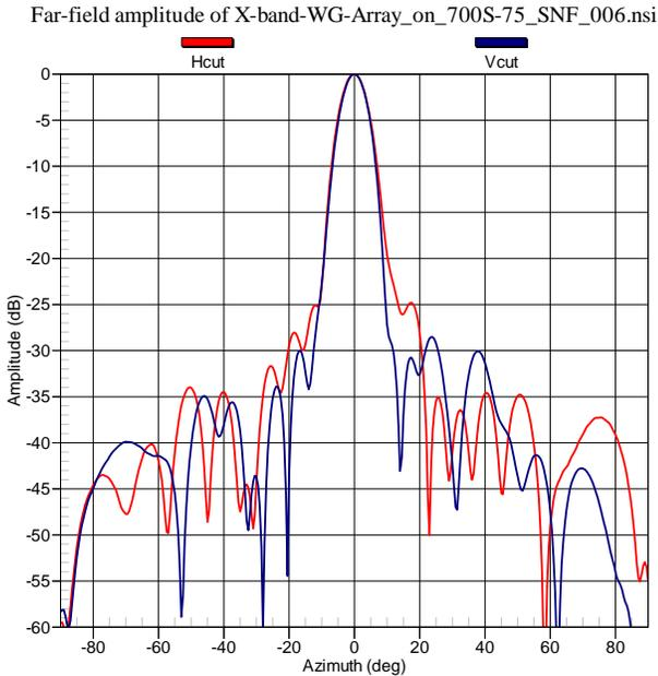
**Figure 3**– X-band Waveguide Array on NSI-700S-75 SNF Scanner
