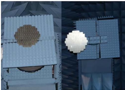
**Figure 7** – X-band Waveguide Array Antenna at centered and lateral offset positions
