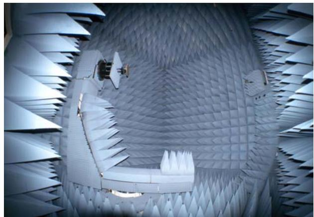
**Figure 1**– X-band Waveguide Array on NSI-700S-75 SNF Scanner
