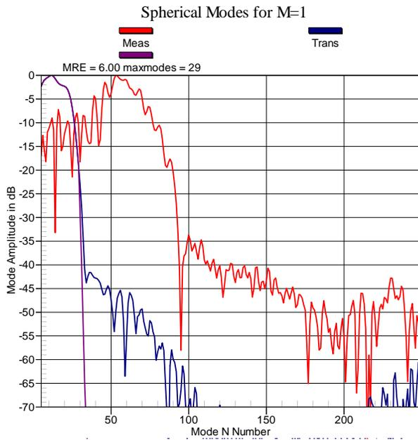
**Figure 10** – Spherical Modes and MARS Filtering Example
