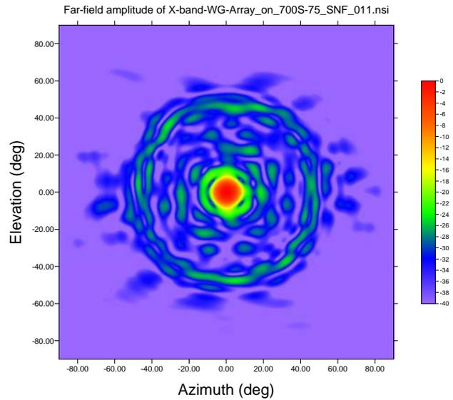
**Figure 4**– Far-field pattern with metal plate obstruction
