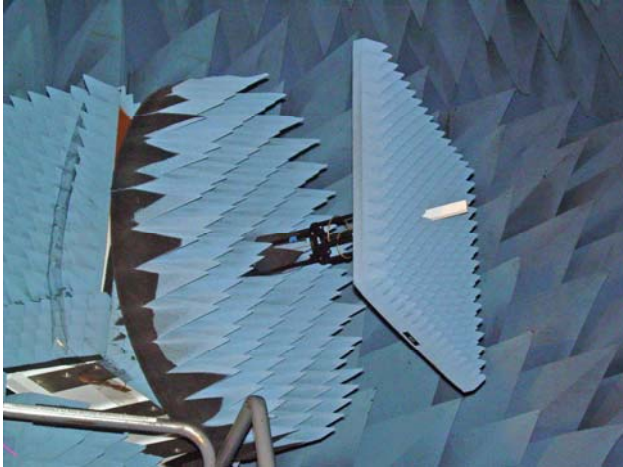
Figure 2 - WR90 OEWG probe with 24 X24 in absorber collar.
