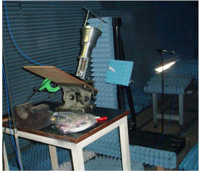
Fig. 2 X-band corrugated horn shown being aligned on QMUL NSI-200V-3x3 combination planar/cylindrical system.
