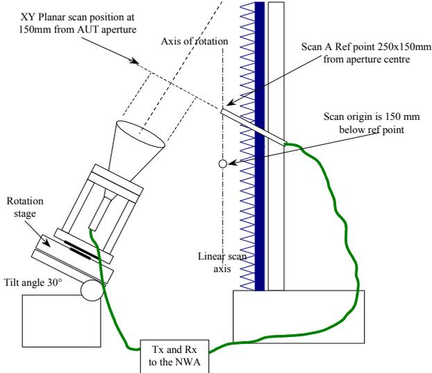
Fig. 3 Schematic of frustum measurements as taken using NSI-200V-3x3 combination planar/cylindrical system.
