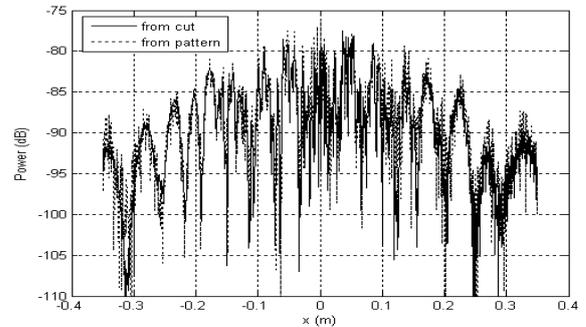
Fig. 4 Comparison of reconstructed normal field component recovered from full two-dimensional pattern and a single cut.
