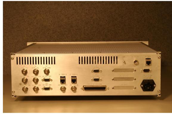
**Figure 4 The MI-788 Networked Acquisition Controller Rear Panel**
