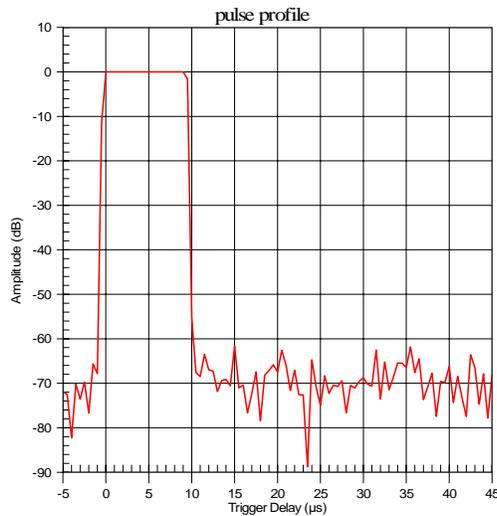
**Figure 9 Panther 9100 Pulse Profile Measurement**
