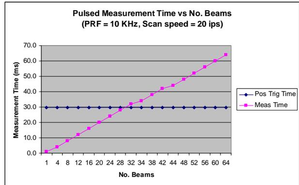
**Figure 4 Measurement Time vs. No. of Beams (PRF=10 kHz, scan speed = 20 ips)**
