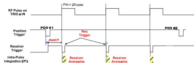
**Figure 7 Pulse Timing (No Intra-Pulse Averaging)**
