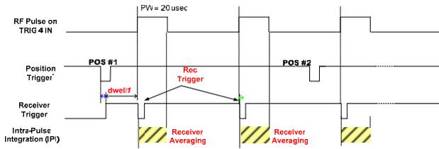
**Figure 8 Pulse Timing (Intra-Pulse Averaging)**
