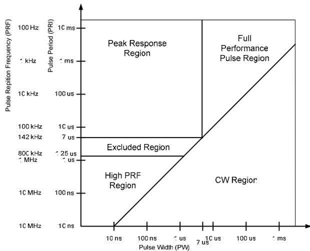
Figure 1 Panther 6000 Pulse Performance Diagram
