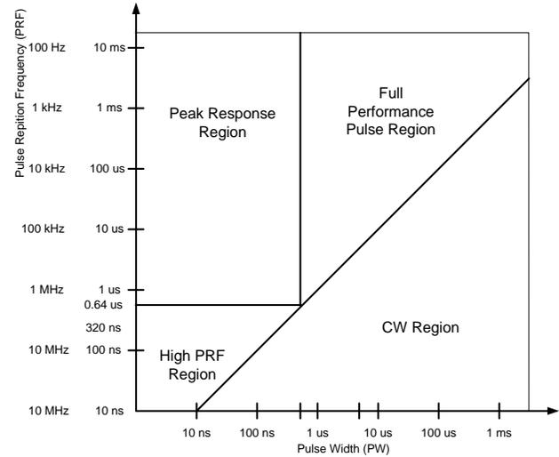
Figure 2 Panther 9000 Pulse Performance Diagram
