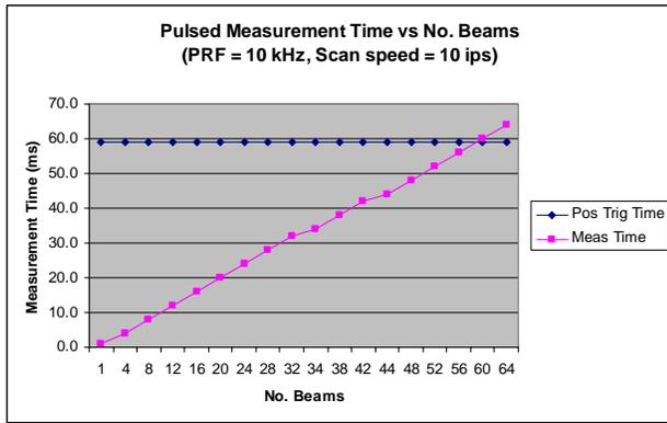
**Figure 5 Measurement Time vs. No. of Beams (PRF=10 kHz, Scan speed = 10 ips)**
