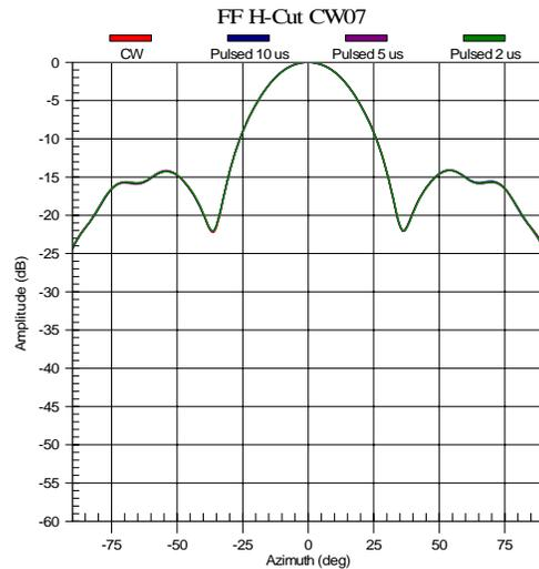
**Figure 10 Pulse vs. CW Comparison**
