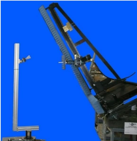
**Figure 7 – Conical Near-Field Measurement System.**
