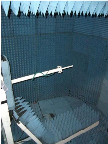
Figure 14 – Omni antenna on NSI-700S-60 SNF
