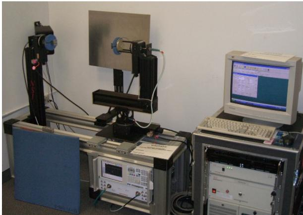
Figure 11 - NSI-700S-20 SNF scanner in NSI conference room with metal plate interference, testing 4-40 GHz ridged horn antenna
