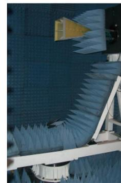
**Figure 8 - NSI-700S-60 SNF scanner in anechoic chamber testing 0.5-6 GHz dual pol horn antenna**
