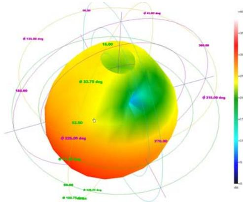
**Figure 5-1 Radiation pattern – 3D view**
