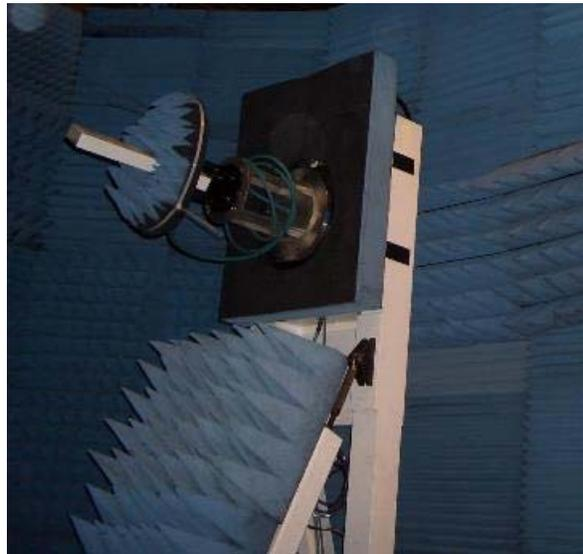
**Figure 4 – NSI-RF-WR284 OEWG probe being tested at NSI on NSI-700S-60 Spherical NF in anechoic chamber**
