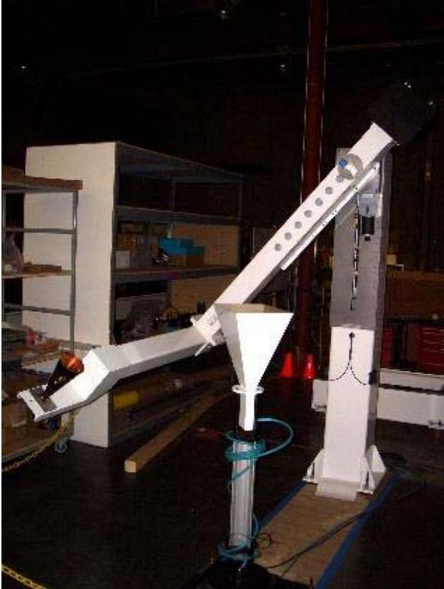
**Figure 9 – NSI-RF-SG284 Standard Gain Horn tested on NSI ARCH scanner with no absorber or chamber**
