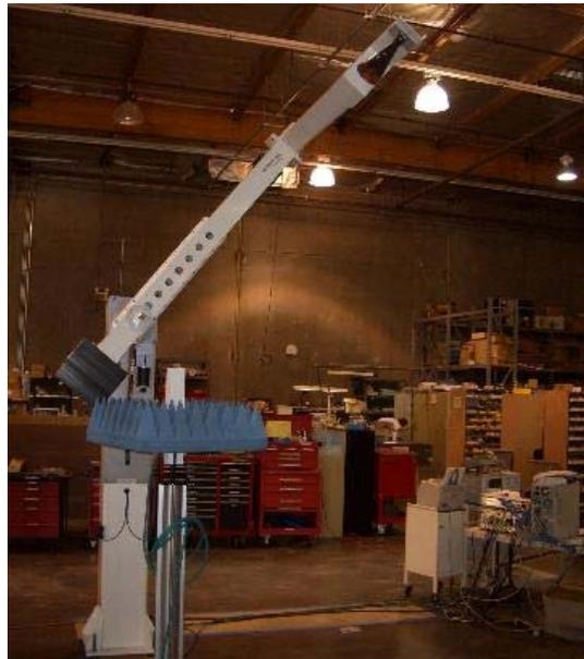
**Figure 5 – NSI-RF-WR284 OEWG probe being tested at NSI on NSI-700S-90 ARCH Spherical NF in open environment with NO anechoic chamber**
