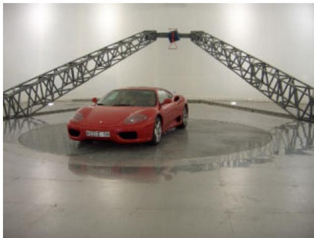
Figure 2 – NSI rotator and gantry testing automobile
