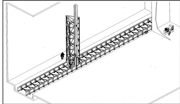
*Figure 6 35m x 16m Vertical Planar Scanner*
