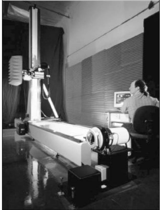
*Figure 3 4m X 3m Vertical Planar Scanner*
