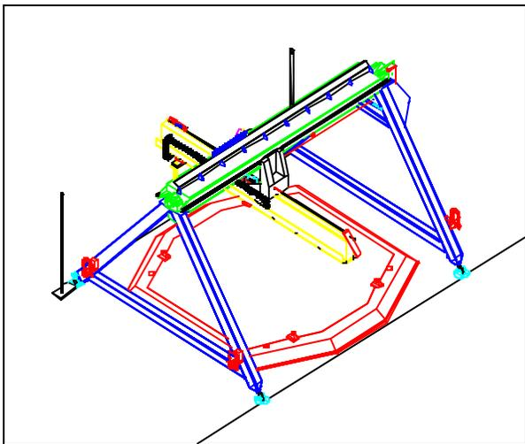
*Figure 13 Planar NF Scanner Used For Testing Aegis Antennas*
