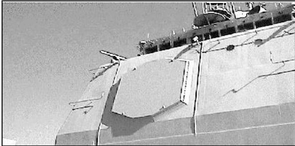
*Figure 12 Aegis Array On US Navy Destroyer*
