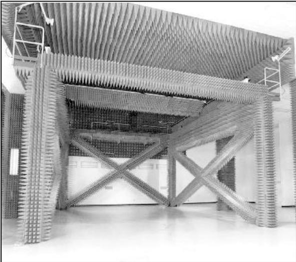
*Figure 9 Hughes 7m X 7m Horizontal Near-Field Range*
