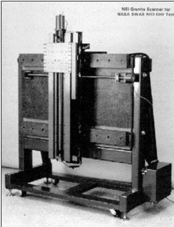
Figure 15 550 GHz vertical planar scanner
