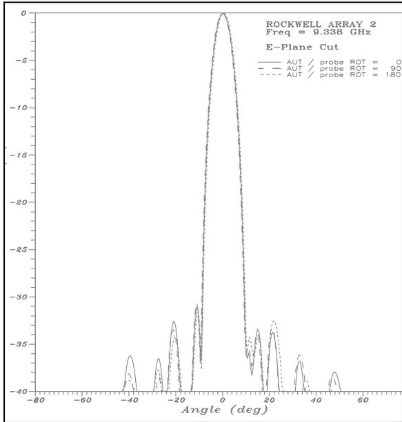
Figure 9 Self Comparison Test 3 Scans @ 0,90,180 Degrees (Multipath Suppressed)
