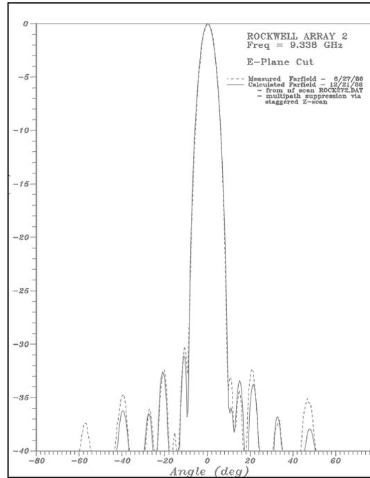
Figure 11 E-plane Cut Near-field vs. Far-field
