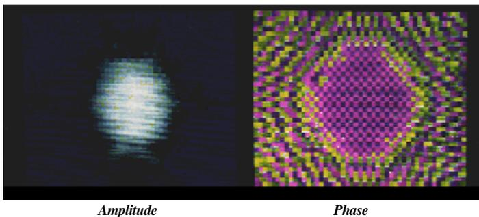
Figure 6 Nearfield Amplitude / Phase
