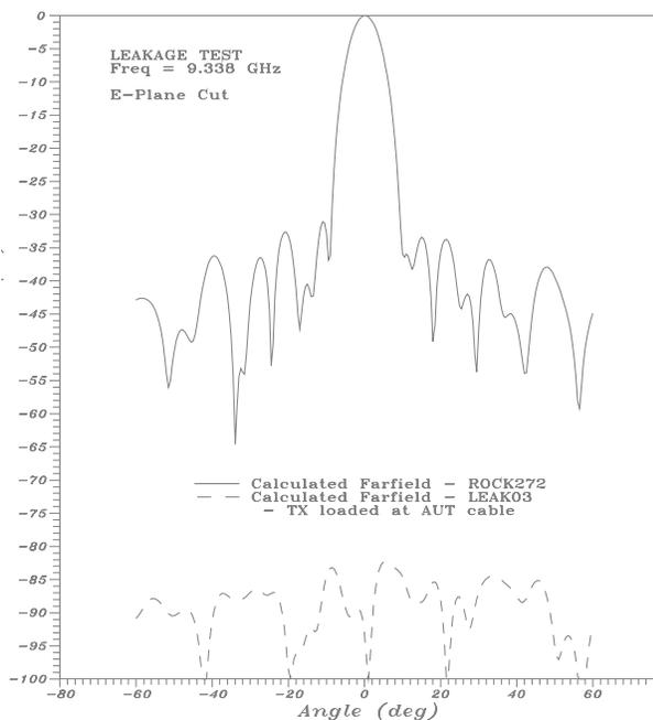
Figure 2 E-Plane Cut / Leakage (AUT Loaded)
