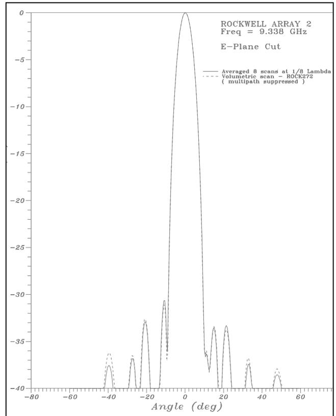
Figure 7 Averaged Result vs. Volumetric Scan
