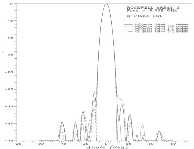
Figure 5 E-Plane Cut vs. AUT/Probe Distance
