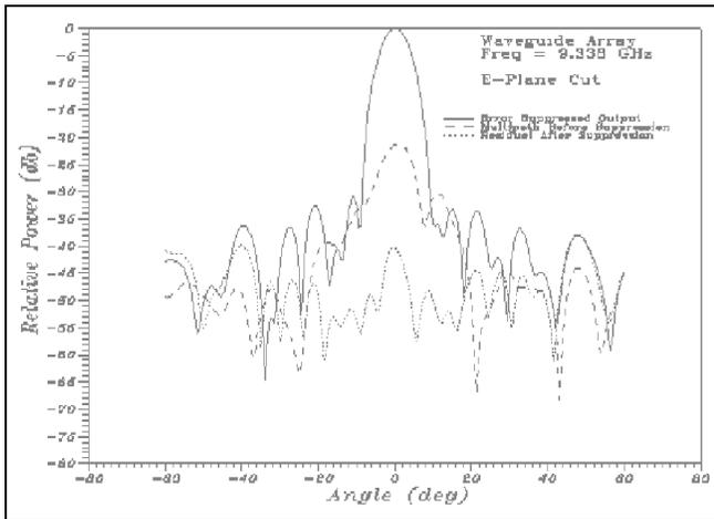
Figure 10 - Multipath vs. Desired Signal
